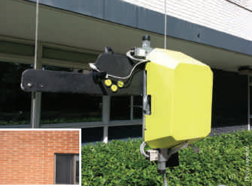
SAM at work – getting ready to inspect and photograph the building envelope. Inset: detail of a photo taken by SAM.
